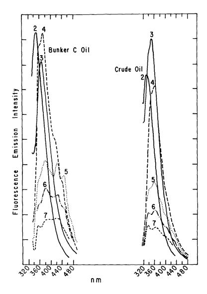
Fig. 1. Fluorescence emission spectra of oil fractions eluted from the alumina column. Each fraction consists of 3 ml effluent. Fraction 1 (first 3 ml after sample application) had emission spectrum of solvent blank. Spectrum of fraction 3 was recorded at 50% sensitivity.
