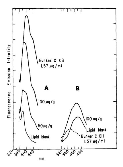
Fluorescence emission spectra of herring lipid, spiked with Bunker C oil. Fig. 2. A - cleaned-up extracts, B - extracts without cleanup.
